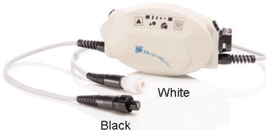
**Figure 5** HeartMate II LVAS System Controller with Leads (note black and white connectors)
