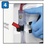
Place the pressure chamber into the pressure chamber well and press the infuse line into the air detector
