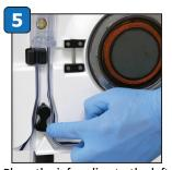
Place the infuse line to the left of the valve wand and the of the valve wand
