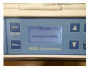
The bed is zeroed successfully and ready for a patient when the screen displays 0.0 lb/kg.
