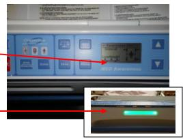
If any of the parameters you set change, the light on the footboard will blink amber and the screen will tell you exactly what parameter has changed. Fix that parameter to make the light go green again.
